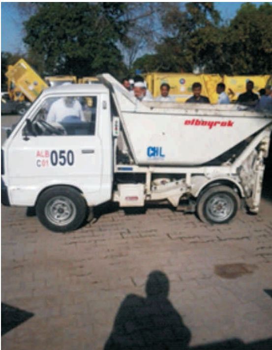
Suzuki pick up mounted 1 m 3 dumper (manual loading and mechanical unloading)
