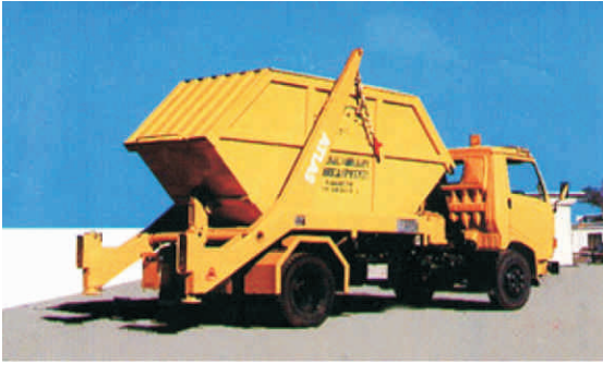
Figure 1.7: Hoist truck with 7 m 3 container loaded on it
