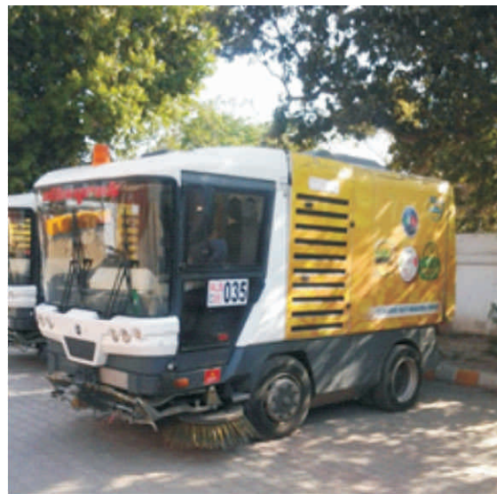
Mechanical sweeper 4 m 3 capacity
