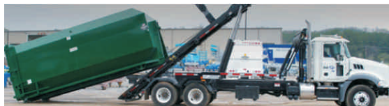
Figure 4.6: Collection vehicle used to haul and empty large containers (2 to 10 m 3 ). Container hoist and unloading mechanism is mounted on truck frame [2].
