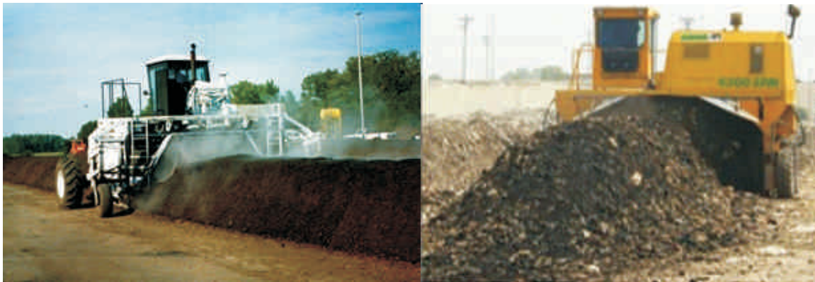
Figure 7.5: Specially designed machines used to turn composting material placed in windrows
