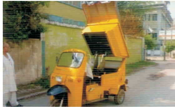
Figure 1.4 (a): Locally manufactured Auto Tri-Wheeler with manual loading and mechanical unloading arrangements
