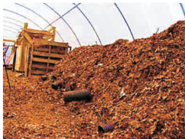
Figure 7.7: Passively aerated windrow
