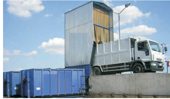
Fig. 5.7(b): stationary compactor-container transfer station
