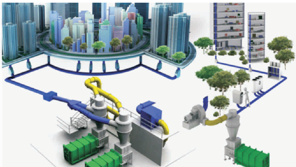
Figure 5.10 (a): Stationary pneumatic collection system [8]
