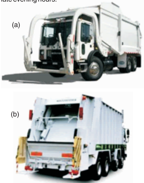
Figure 4.4: Self-loading collection vehicle equipped with internal compactor: (a) front loader (b) rear loader [2].
