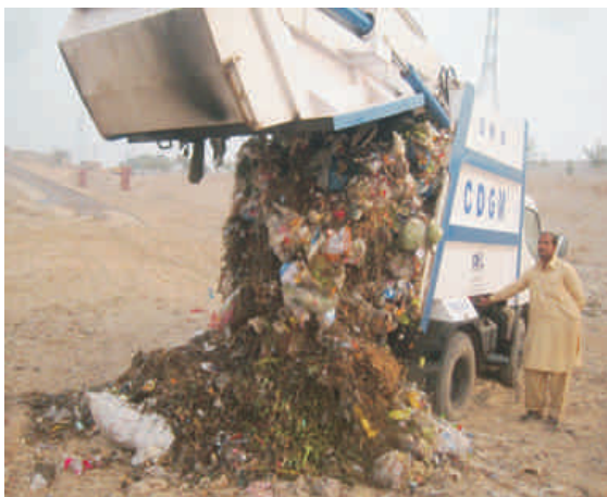
Figure 8.22: Unloading of collection vehicles
