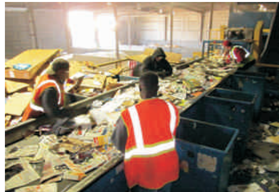
Figure 6.9: (a) Conveyor assisted sorting
