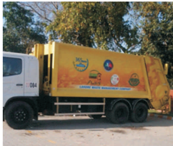
Compactor truck, 6 m 3 capacity used by LWMC
