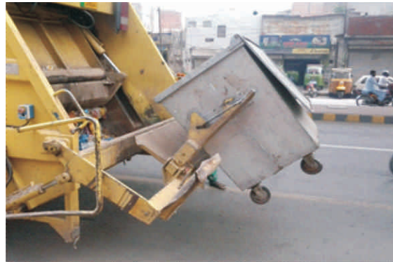
Figure 4.10: Mobile mechanical waste compactor for waste collection [3].
