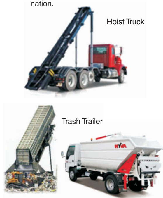
Figure 5.8: Vehicles used for the transportation of solid waste
