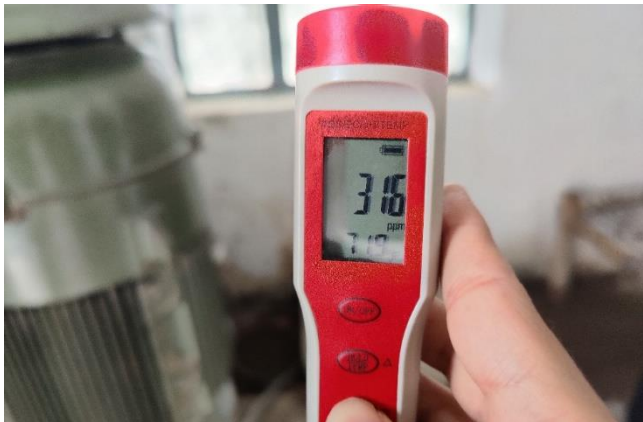
TDS value of 316 ppm was observed during Rapid Water Quality Testing. Pakpattan is blessed with sweet groundwater (average TDS values 286 ppm) with water table on average being 70-80 ft.
