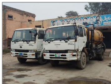
Existing Sucker & Jetting Machines
