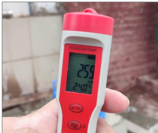
Rapid Water Quality Testing at the source (TDS: 259 ppm)
