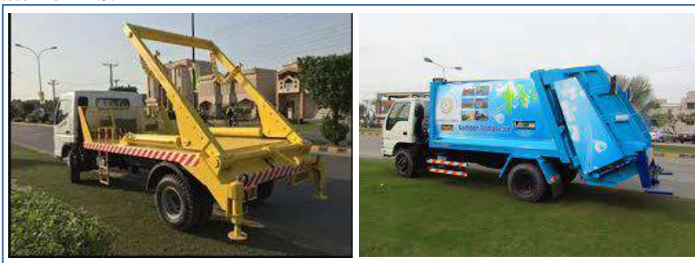
Figure 3.3: Secondary Container lifting Vehicles
