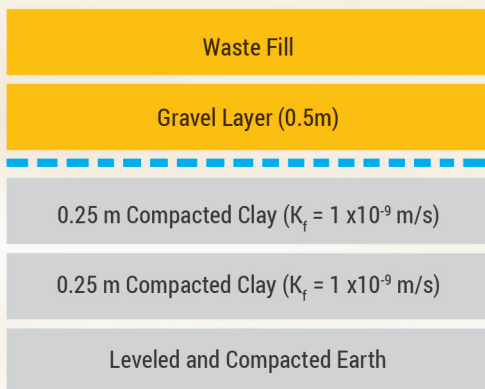
Base Sealing System of the Lakhodair Landfill Site
