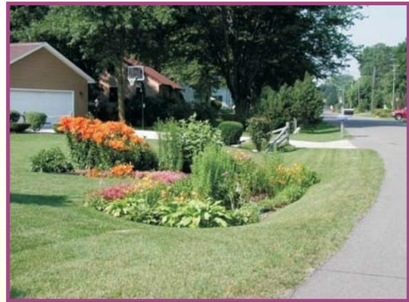
A soil storage and rainwater seepage system
